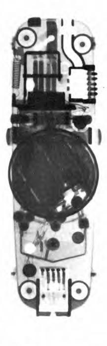
RADIOGRAPH, left, provides a different image from x-ray, right. Various components of Princess telephone base are visible in one and not in the other. Because of sensitivity to carbon and plastics, Division 7361 uses radiographs in nondestructive testing of items using these materials.
